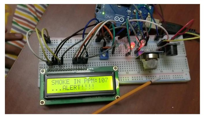
When smoke is detected by the sensor red LED will glow.
